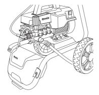
8- Connect the high pressure hose to the trigger gun.
